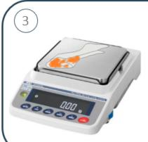
Weigh the cloth with the grease wiped off, subtract the cloth weight and compare the result with a reference value of 30 g.
